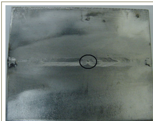
a) Photograph of welded joint with lack of fusion defect
