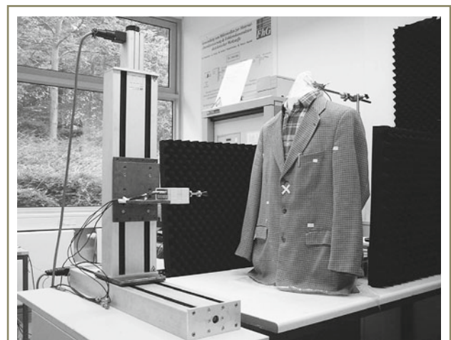
Figure 10 – Mechanical two-axis-scan of objects concealed under a jacket with FMCW-radar
