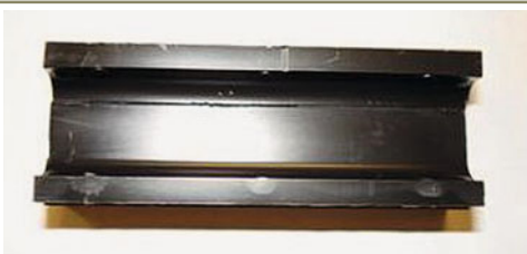
a) Just welded sample
