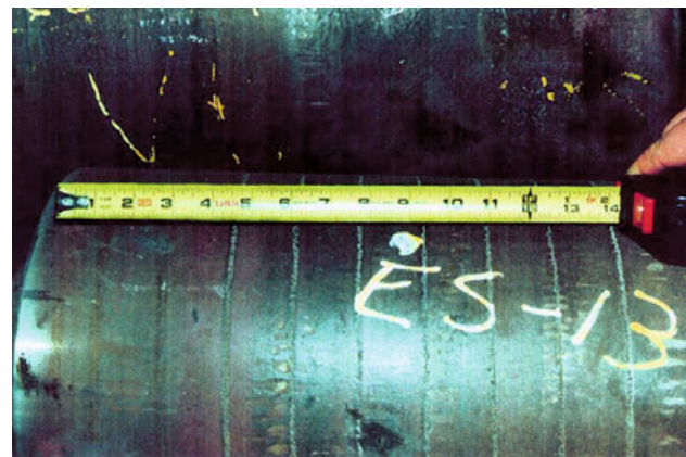
Figure 3 – Inter-bead corrosion of a continuous casting roll surface
