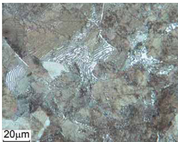
Figure 2 – Fully pearlitic microstructure of the base material (eutectoid steel)
