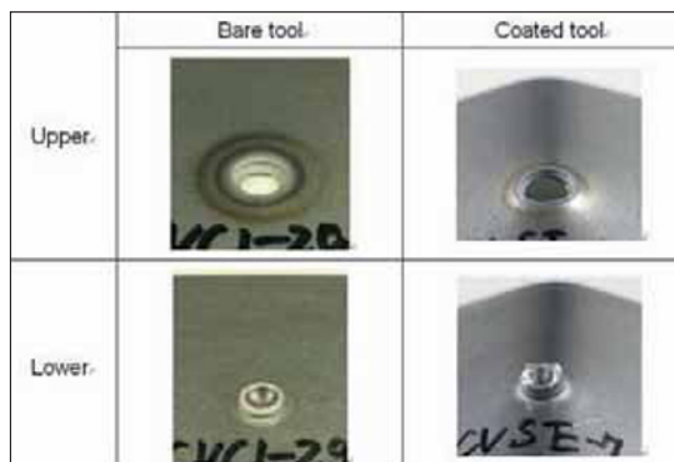
Figure 8 – Appearance of fracture parts after cross tension test
