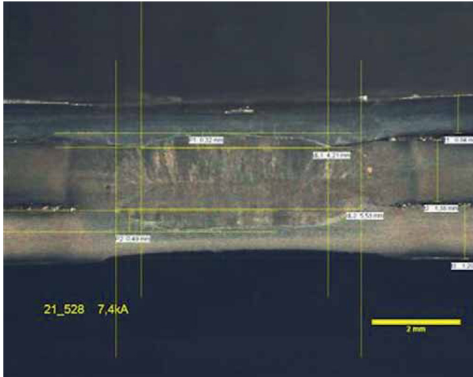
Figure 15 – Cross section analysis of a 3-sheet metal stack-up indicating sheet thickness, nugget diameter and weld penetration depth
