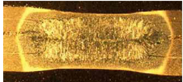
b) Cross section through a spot weld with 7.0 mm diameter and moderate electrode indentations
