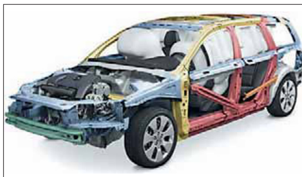
Figure 1 – The safety cage structure of the new Volvo V70 model and the function of the supplementary restraint systems (SRS); frontal air bags (FAB) and inflatable curtains (IC)
