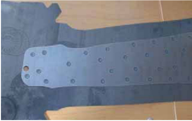
a) Upper control hole for exact positioning of the patch blank
