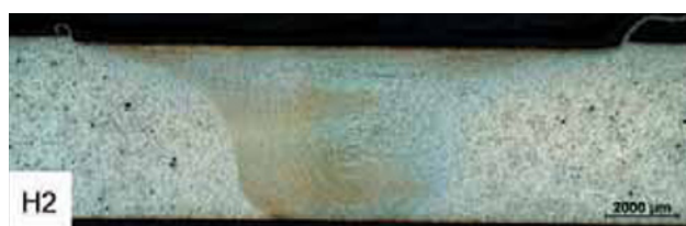
a) Weld produced with a weld gap of 0.2 mm
