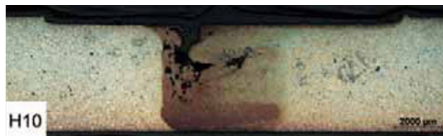
e) Weld produced with a weld gap of 1.0 mm
