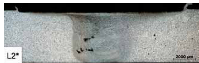
b) Weld L2*(executed with higher plunge depth and 0° tilt angle instead of 2°)
