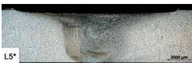
a) Weld L5* (weld gap of 0.5 mm)
