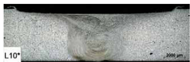
b) Weld L10*(weld gap of 1.0 mm)
