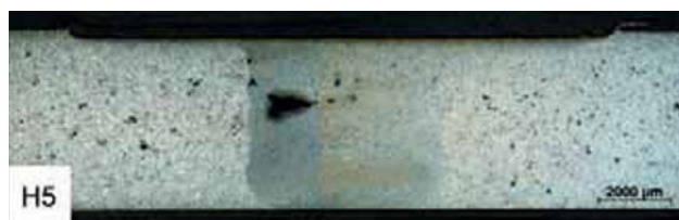
c) Weld produced with a weld gap of 0.5 mm
