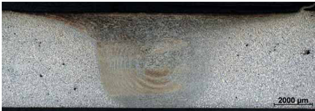
Figure 10 – Etched macrograph of a typical friction stir weld in EN AC-46000 (corresponding with weld E in Table 3)
