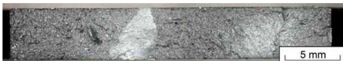
Figure 4 – Fracture surface of a tensile test specimen in EN AC-46000 base material
