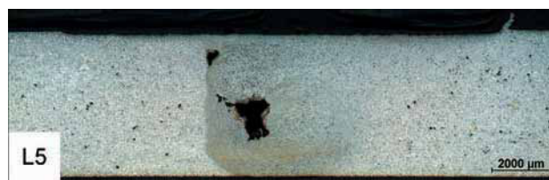
d) Weld produced with a weld gap of 0.5 mm
