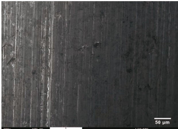
Figure 9 – Topography of sample surface prior to wear resistance test, magnification 300x [13]
