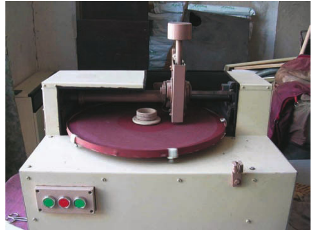
Figure 8 – Equipment for abrasive wear test [12]
