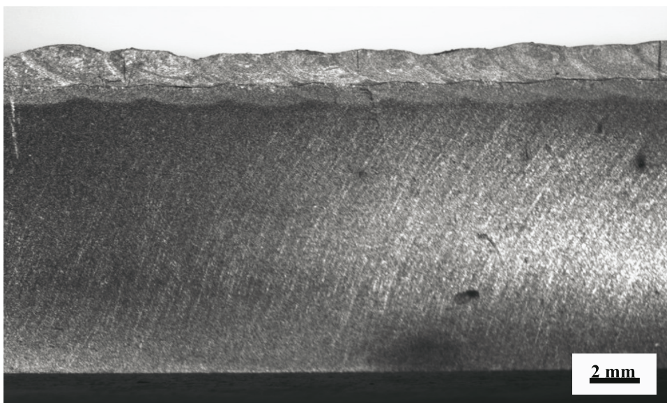
Figure 2 – Macrostructure of sample No. 11, CS 52 powder [10]
