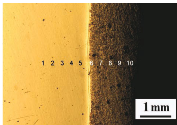
Figure 5 – Structure of laser weld overlay of CS52+30\% (TiB_2-CrB_2) with marked points of analysis [3, 5, 9]
