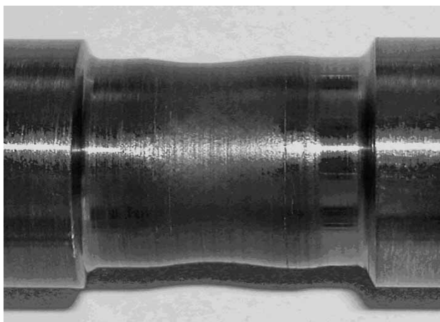
Figure 3 – Mid-portion of the all-weld metal, sample after the ACT, run till drop of the initial material strength to one-third
