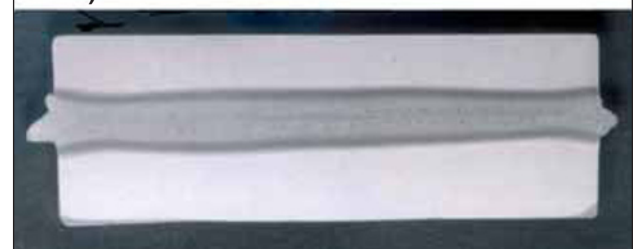
a) 200 kV 60 kW beam in helium at 5 mbar
