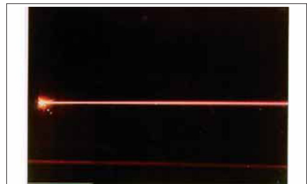
a) 200 kV 60 kW beam in helium at 5 mbar
