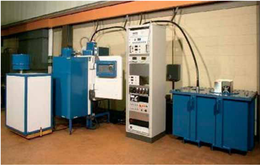
Figure 22 – 150 kV, 8 kW high intensity EB machine
