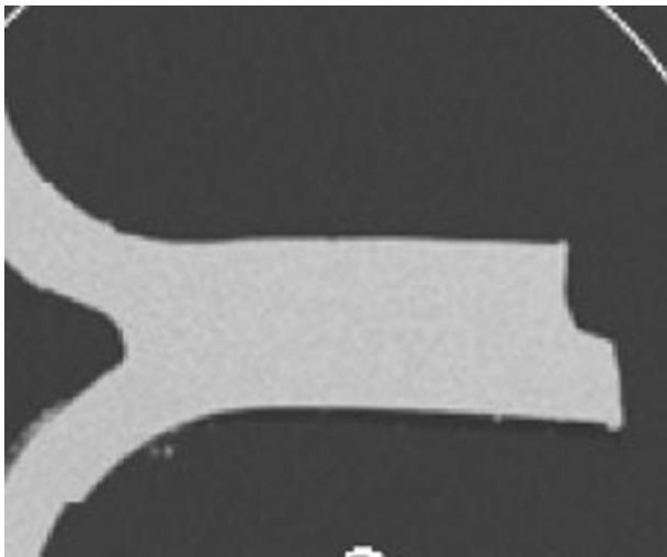
c) Joints made of 304LN stainless steel and brazed with MBF-51 foil
