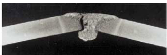
Defect in a single layer weld (MAG), welded on a cooled copper bar.
