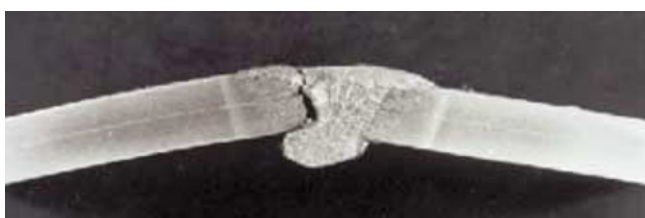
Defect in a single layer weld (MAG) and peaking.
