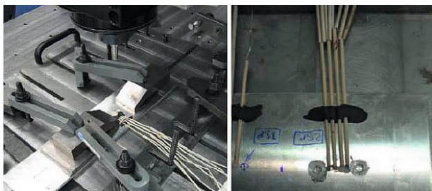
Figure 13 – Thermocouples physical locations between two spots [21]
