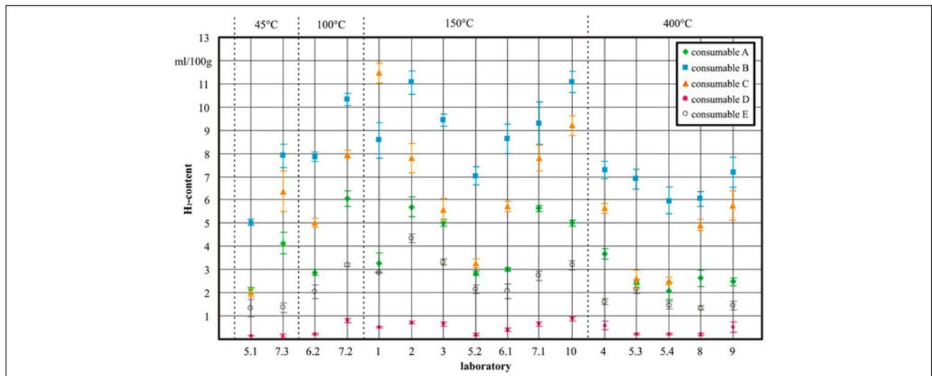
**Figure 2 – Average values and standard deviations in individual test series of laboratories 1 to 10 for consumables A to E**
