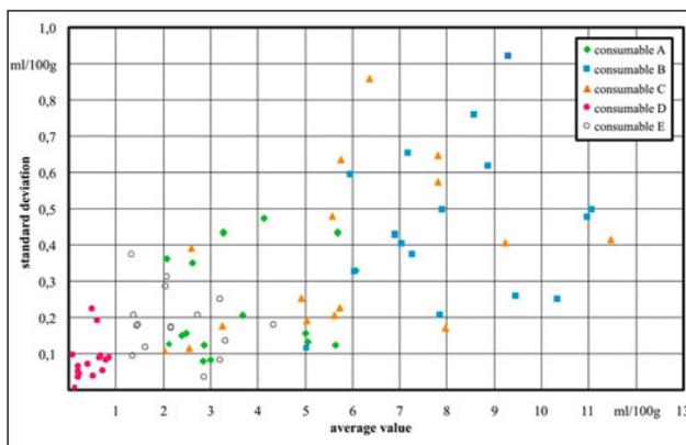
**Figure 3 – Absolute standard deviation versus average value of hydrogen content**
