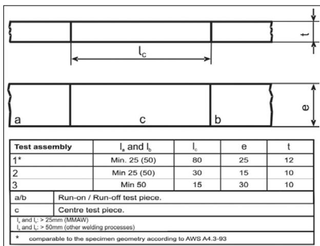
**Figure 1 – Possible specimen geometries according to ISO/DIS 3690 [1], ANSI/AWS A4.3-93 [3], respectively**
