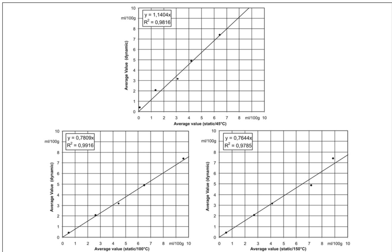
Figure 9 – Comparison between static and dynamic measurement techniques for various degassing temperature
