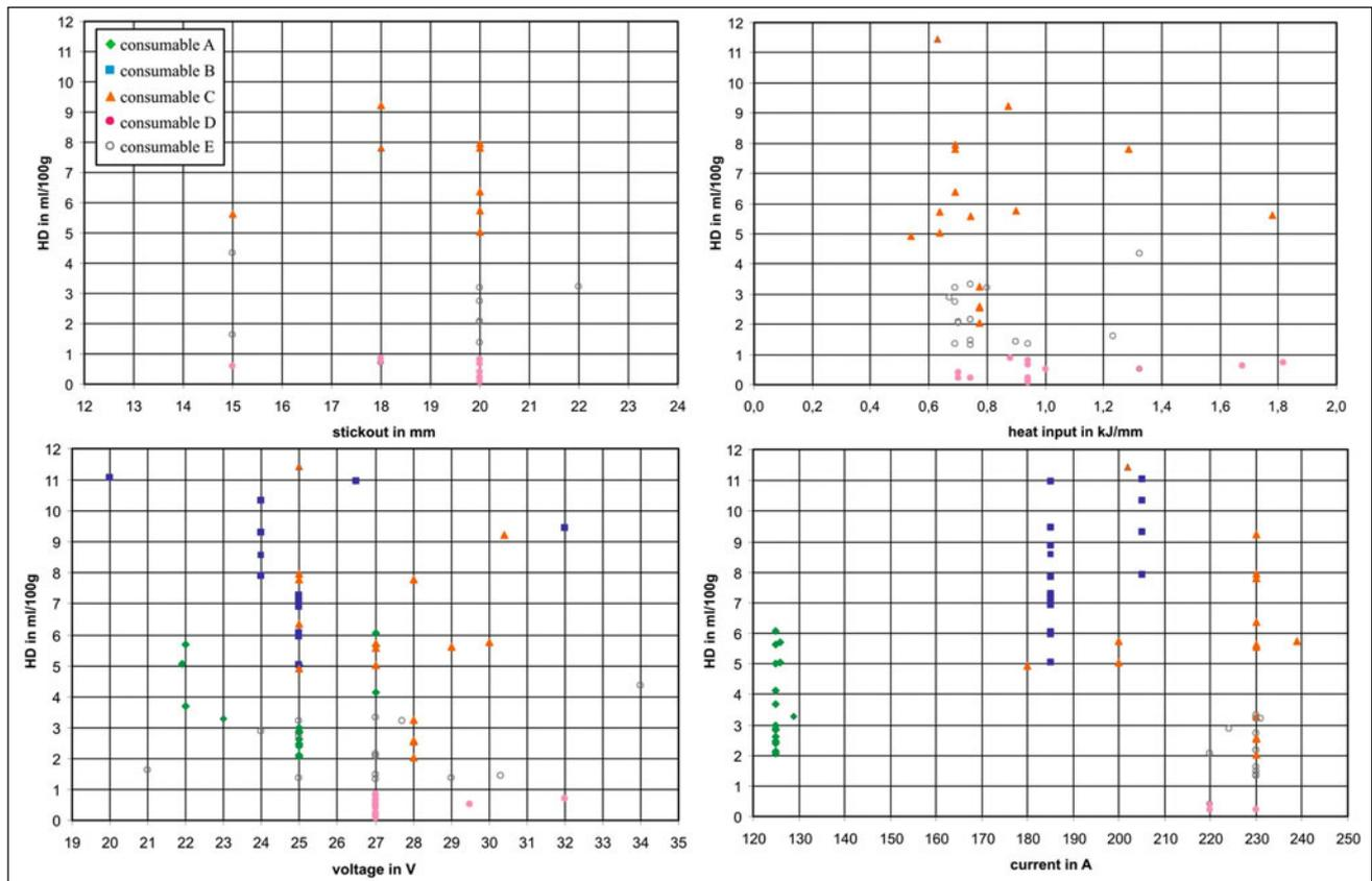
Figure 5 – Diffusible hydrogen content depending on welding parameter
