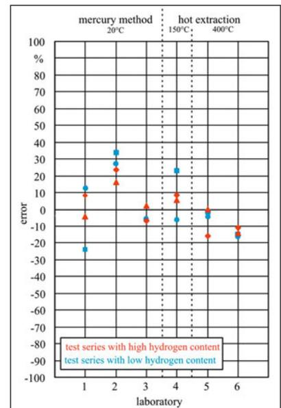
Figure 8 – Relative laboratory-specific error of total average of national round robin test [2]
