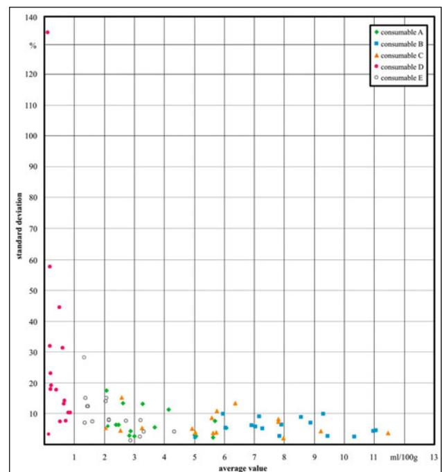
**Figure 4 – Relative standard deviation versus average value of hydrogen content**
