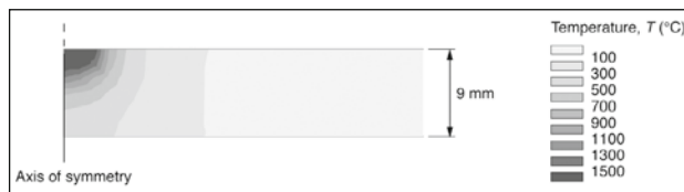
Figure 15 – Isotherms of the welds
