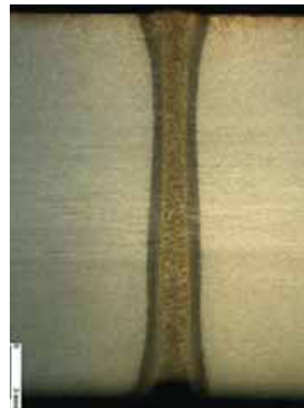
Figure 4 – Single pass welding of 20 mm thick material with an autogenous laser process
