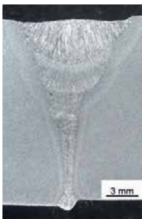
Figure 15 – Cross-section of a hybrid welded sample with 0.5 mm gap and 0.5 mm linear misalignment
