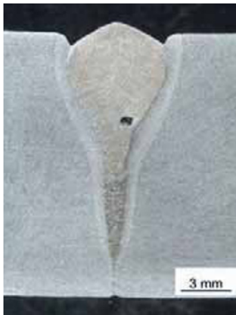
Figure 12 – Cross-section of a hybrid welded sample with 0 mm gap
