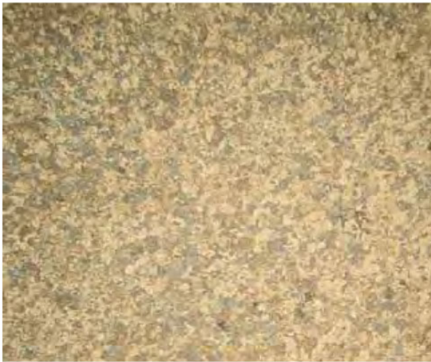
a) Equiaxial grain (magnification: X 200. Etching: Poulton's mod.)
