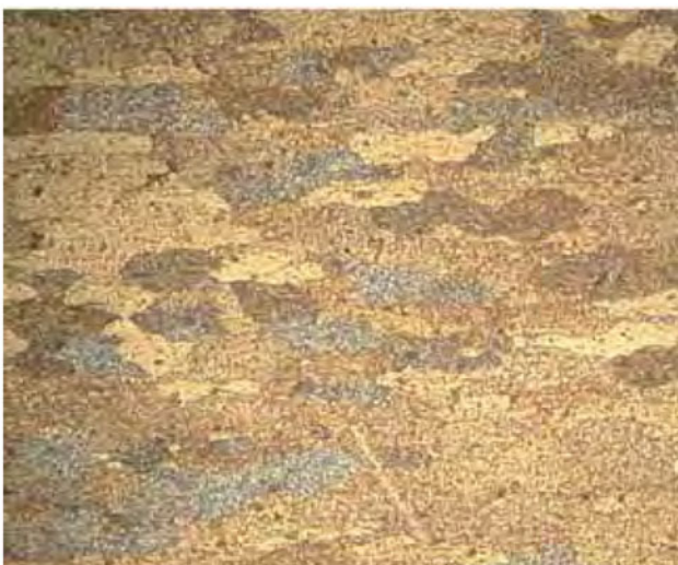
a) Elongated grain (magnification: X 200. Etching: Poulton's mod.)
