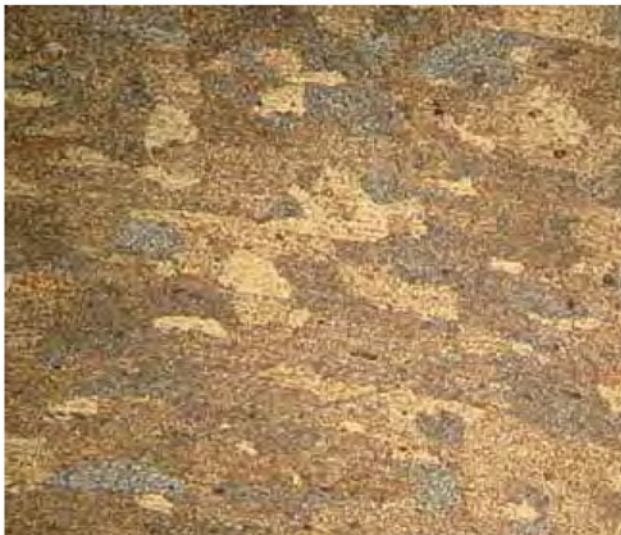
a) Elongated grain plastically deformed (magnification: X 200. Etching: Poulton's mod.)
