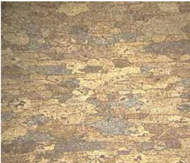
a) Elongated grain (magnification: X 200. Etching: Poulton's mod.)
