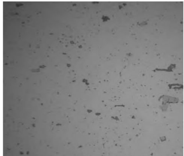
b) Precipitated transgranular (magnification: X 500. Etching: Fluoridic acid)
