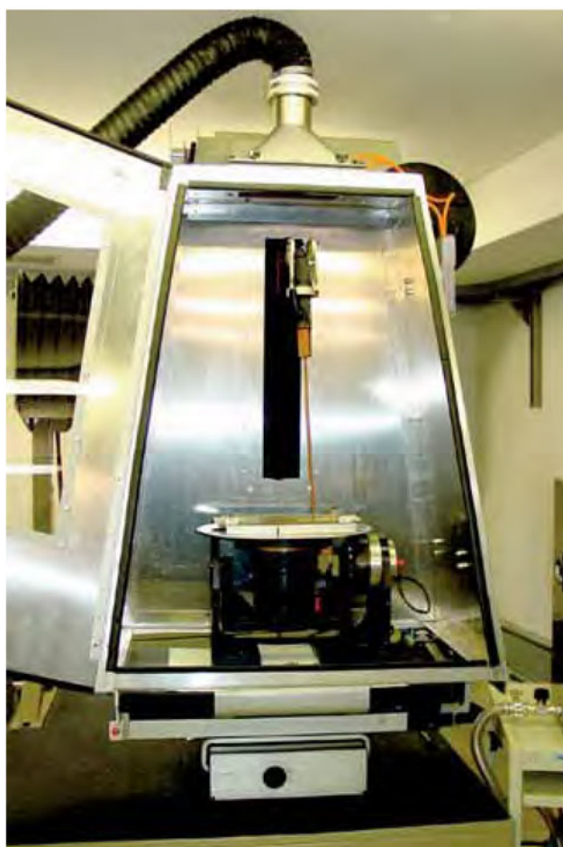
a) Fume collection hood, electrode feed system, and rotary positioning system
