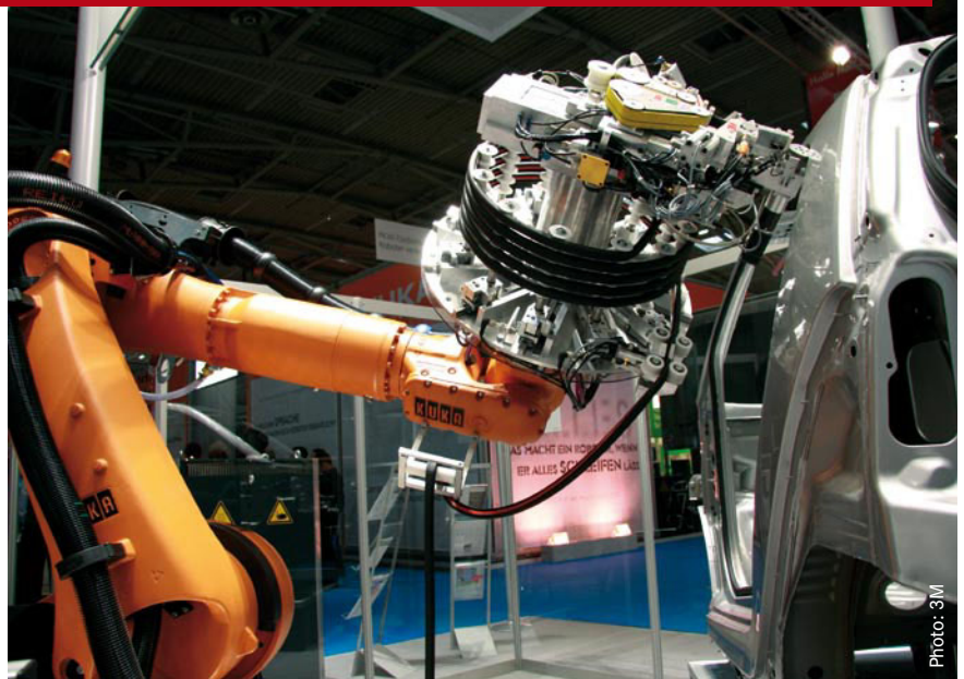
Using a robot, the new application system bonds the seals to the bead on the bodywork.
