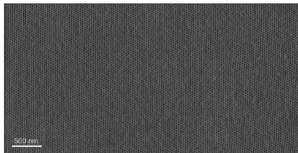
Figure 16. Long range ordering of cylindrical microdomains of PEO in PS- b -PEO thin films annealed in a benzene vapor. Reproduced with permission from Ref. 356; Copyright 2004, WILEY-VCH Verlag GmbH & Co. KGaA.
