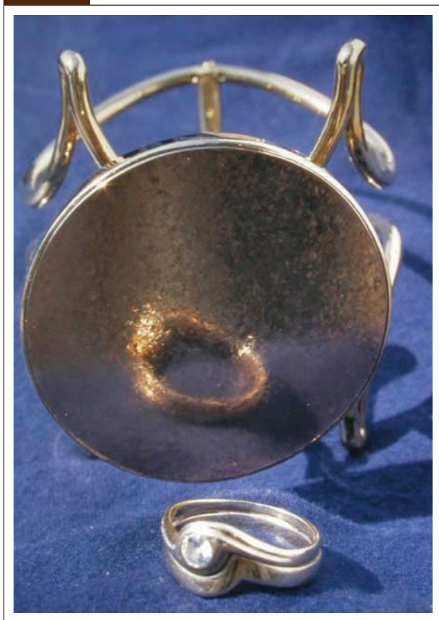
The textured effect produced by a martensitic transformation on the planar surface of a Spangold "tension bangle" is evident in the reflected image of the ring. (Tension bangle designed and manufactured by jeweller Kurt Donau of Johannesburg, South Africa for exhibition at the 1993 Basel Watch and Jewellery Fair in Switzerland. This work was financially supported in 1993-94 by the World Gold Council and Mintek, South Africa. Photo: M.B. Cortie and F.C. Levey)
