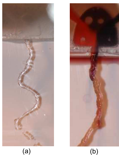
Fig. 6. Water visualization of the fluidic oscillator at a supply pressure of 1.8 psi.
