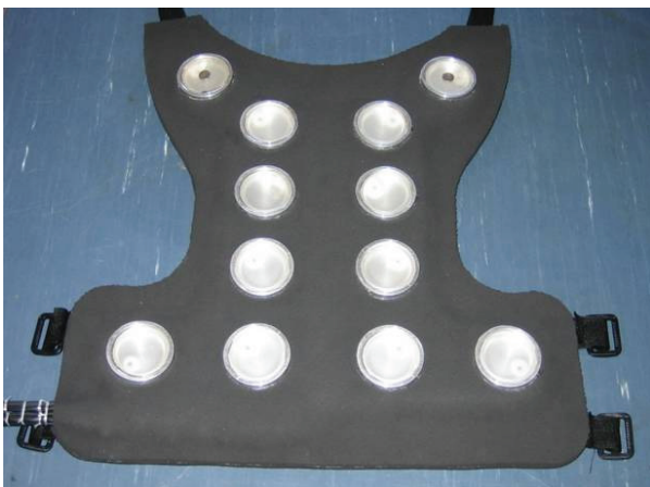
Figure 5. Posterior chest wall part of the jacket to record lung sounds.
