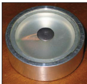
Figure 7. ECG lead built into the diaphragm of an electronic stethoscope.
