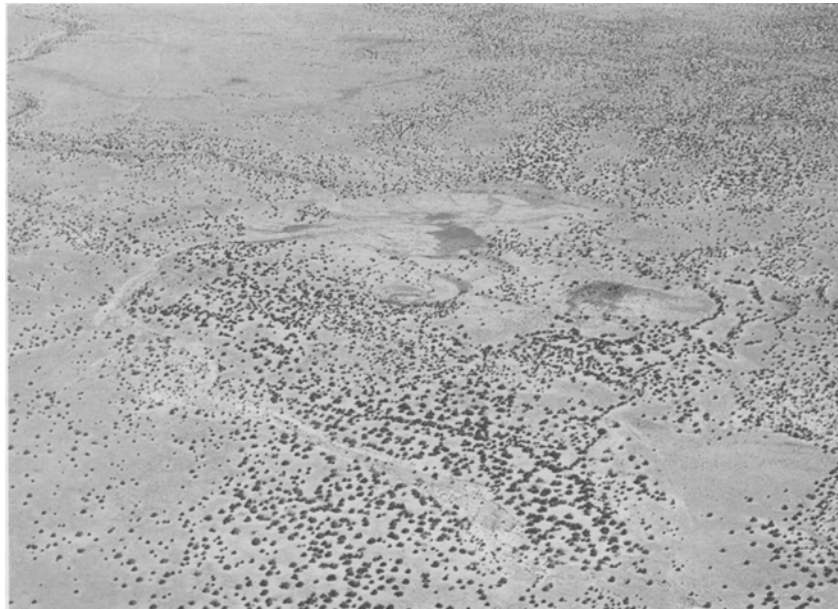
Figure 7. Richard Lake depression (center) with sinkhole sump in very center, occupying lowest elevation. Semi-concentric buckles are visible at right; linear buckle outlined by junipers at near side of depression is parallel to trend of Holbrook Anticline extension.
