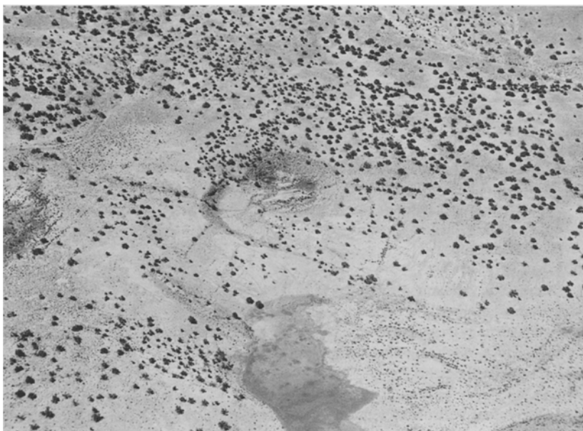
Figure 9. Aerial view showing 170 m-wide central sinkhole. Buckle folds outlined by linear growth of junipers are visible on all sides of the sinkhole; others trend diagonally across the photo about N 45° W, similar to the trend of the Holbrook Anticline.
