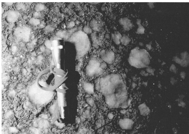
Figure 4. Example of nodular gypsum exposed in Triple Engle Pit. Note relatively pure gypsum nodules encased in muddy carbonate matrix.
