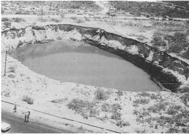
Figure 8. Aerial view of Wink sink in west Texas. The sink, with a diameter of 110 m, formed in 1980 at the site of an abandoned oil well. Photo courtesy of R.W. Baumgardner, Jr.
