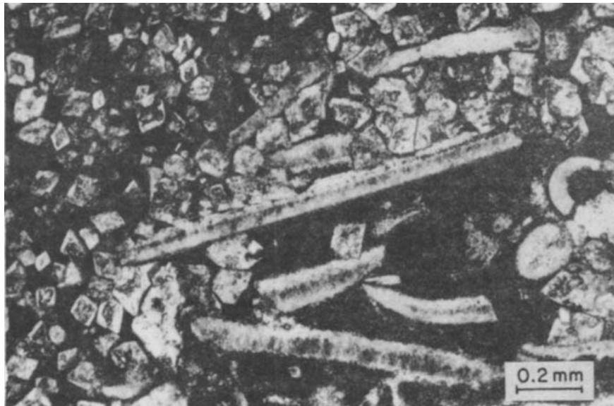
Photomicrograph of skeletal grainstone. Fossil fragments have created shelter porosity. Euhedral dolomite crystals surround allochems. Tribes Hill Formation, Lower Ordovician, Mohawk Valley, New York (Figure 15 on page 236 in Curl, M.W., Zagorski, T.W., and Friedman, G.M., 1984, Depositional environments and diagenesis of subsurface Tribes Hill Formation (Lower Ordovician), Mohawk Valley, New York: The Compass of Sigma Gamma Epsilon, v. 61, p. 216-243).
