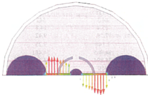
Fig. 4. Cross-sectional profile of rf electric field vectors and energy in a plane perpendicular to the axis of the 10 mm long 3-loop-2-gap resonator obtained for the n = 0 mode by computer simulation. Red to blue indicates maximum to zero intensity.
