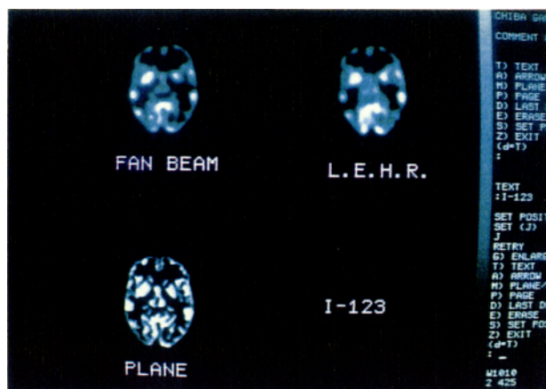
Fig. 5 Images of the “Hoffman Phantom” filled with ^{123}\text{I} solution. SPECT images were reconstructed from 90 views. The acquisition time for each collimator at each step was 30 seconds.
