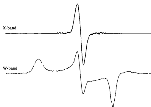
Fig. 6. X-band and W-band EPR spectra of dibenzothiophene (DBT) cation radical, formed by ultraviolet irradiation, in boric acid glass. The magnetic field scan range is 300 Gauss. The X-band spectrum is rescaled from a 100 G scan.
