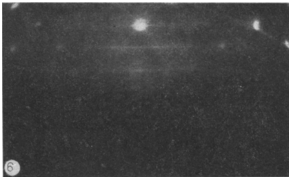
Fig. 6. Electron diffraction pattern of a cleavage surface of a ZnS single crystal
