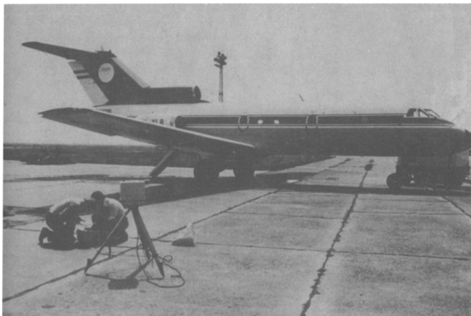
Fig. 3. HPIC in position of field measurement in front of the aircraft used for measuring cosmic dose rates in air at various altitudes
