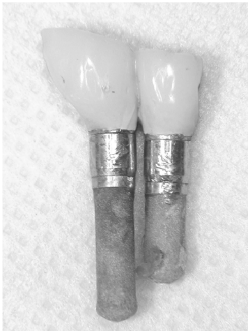
Fig. 5. Retrieved implant complex of Steri-oss system.
