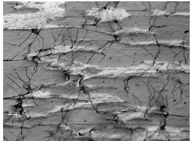
Fig. 10. Optical images taken from the outer surface of the failed BMG composite containing 40 vol.% brass; many shear bands are initiated from the interface between brass-fibers and the matrix, but they do not propagate through the neighboring brass-fibers.
