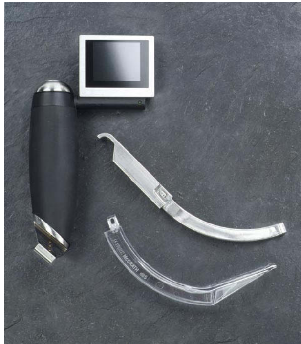
FIGURE 3 The McGrath® videolaryngoscope disassembled, showing the handle and liquid crystal display screen (left), “camera stick” (top right) and a single-use blade (bottom right).
