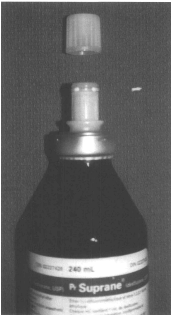
FIGURE Suprane® (Desflurane) refill bottle demonstrating the damaged "O" ring of the SAF-T-FILI™ bayonet fitment.
