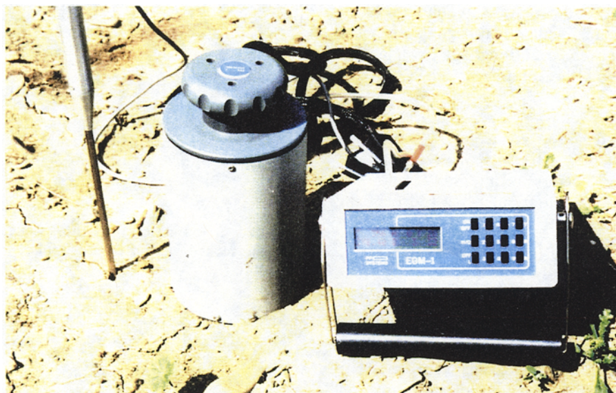
Fig. 3: Soil respiration measurement during soil decontamination showing the portable instrument and respiration chamber
