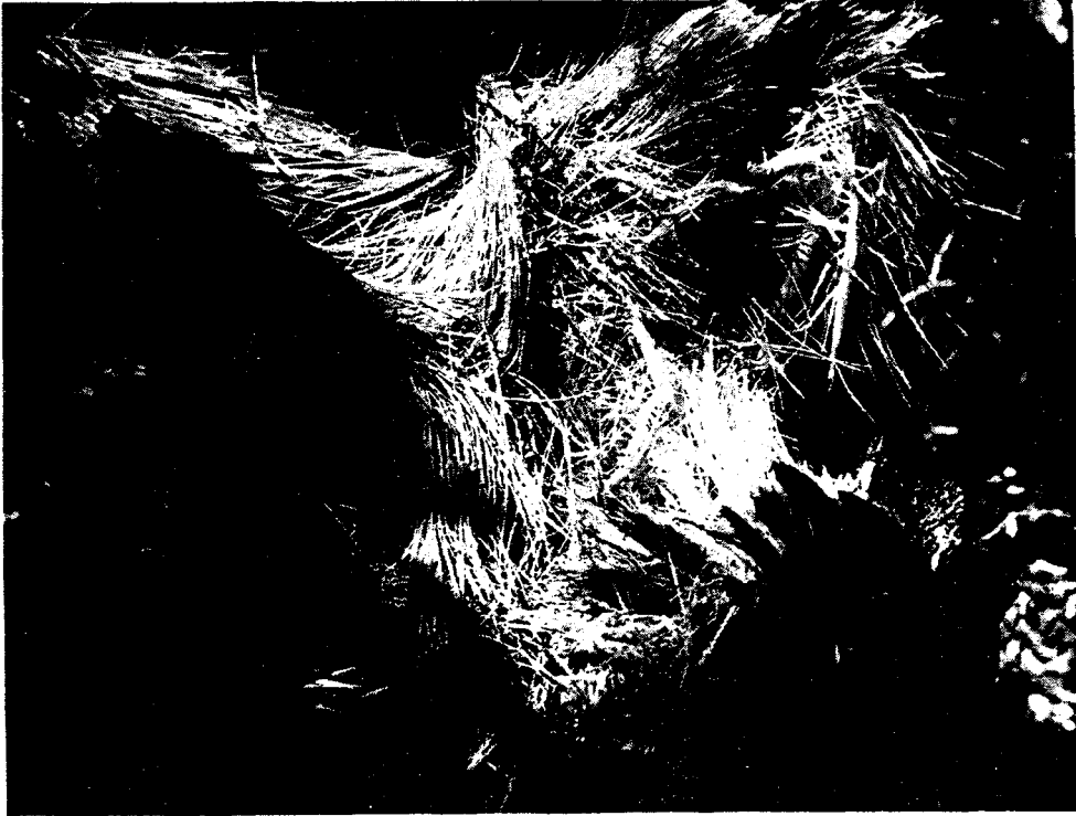
FIG. 12. Longitudinal section of mbocayá palm showing complete destruction except for cellulose fibers caused by snout beetles.
