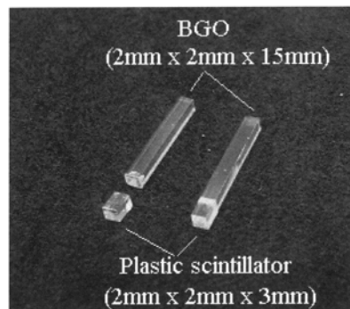
Fig. 4 Photograph of phoswich scintillator, before optical coupling (left) and after optical coupling (right).
