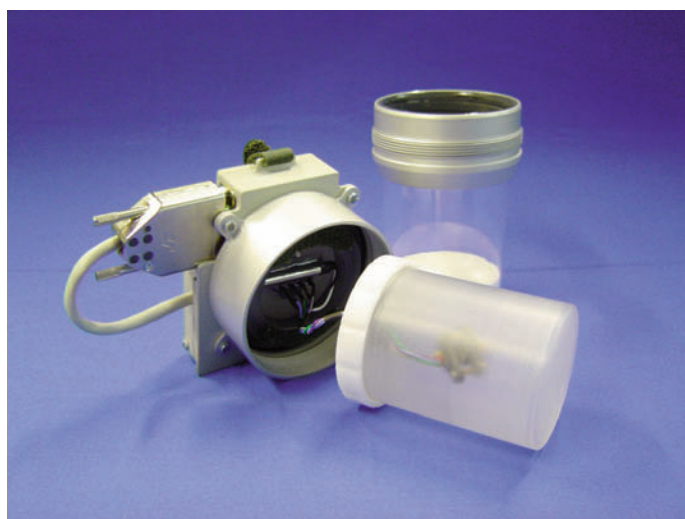
Fig. 2. Disassembled BugNRG experiment facility. Counter clockwise: the experiment-bus also showing the temperature probe, 2nd level of containment and 3rd level of containment
