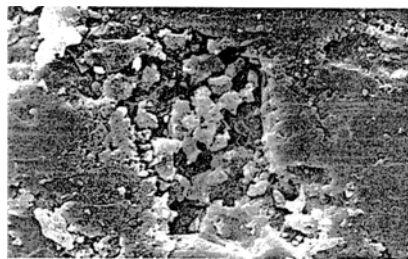
Figure 11 (a) The cross section of plasma-sprayed Ti-6Al-4V/HA coating with (b) evidence of pull-outs during polishing.
