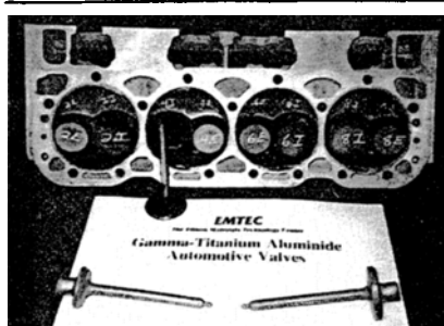
Figure 1. A cylinder head from a road-tested Chevrolet Corvette with the \gamma -TiAl alloy valves.
