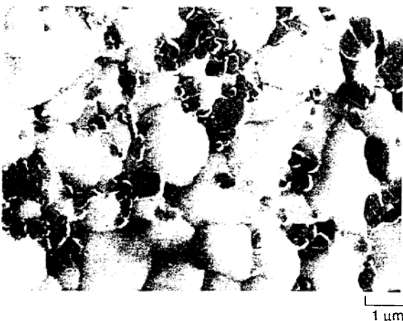
Figure 1. A micrograph of \text{MoSi}_2 -SiC composite processed by displacement reaction and thermally etched. The light areas are \text{MoSi}_2 and dark areas are SiC.
