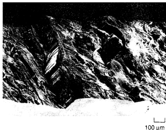
Figure 3. Fatigue fracture morphology of a NiAl-Cr(Mo) composite, revealing the variation of microstructural characteristics and cracking plane.
