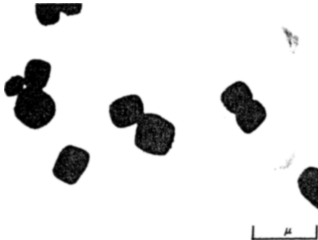
Fig. 3—Extracted \gamma' used for particle size measurements after heat treatment of 1900°F for 27 hr.
