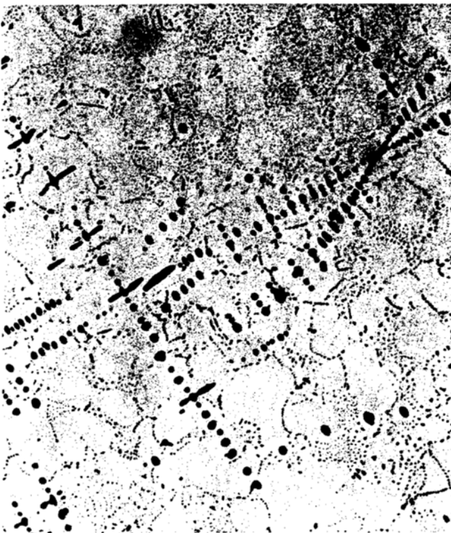
Fig. 7—Alloy 9. Extensive sulfide dendrites, together with Type IIR, formed when manganese is added to a melt at 1547°C, below the freezing temperature of MnS, to put the overall composition in the L + \text{MnS} region. 2.81 pct Mn, 0.72 pct S, Magnification 120 times.
