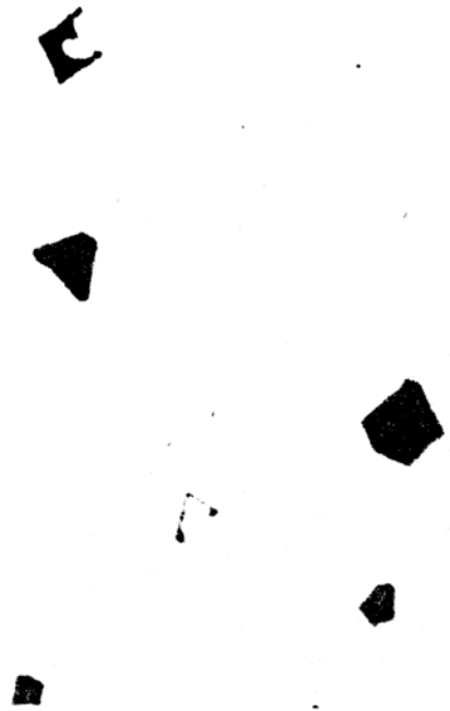
Fig. 15—Type III inclusions in Alloy 34. 2.45 pct Mn, 0.24 pct S, 4.43 pct C, Magnification 600 times.
