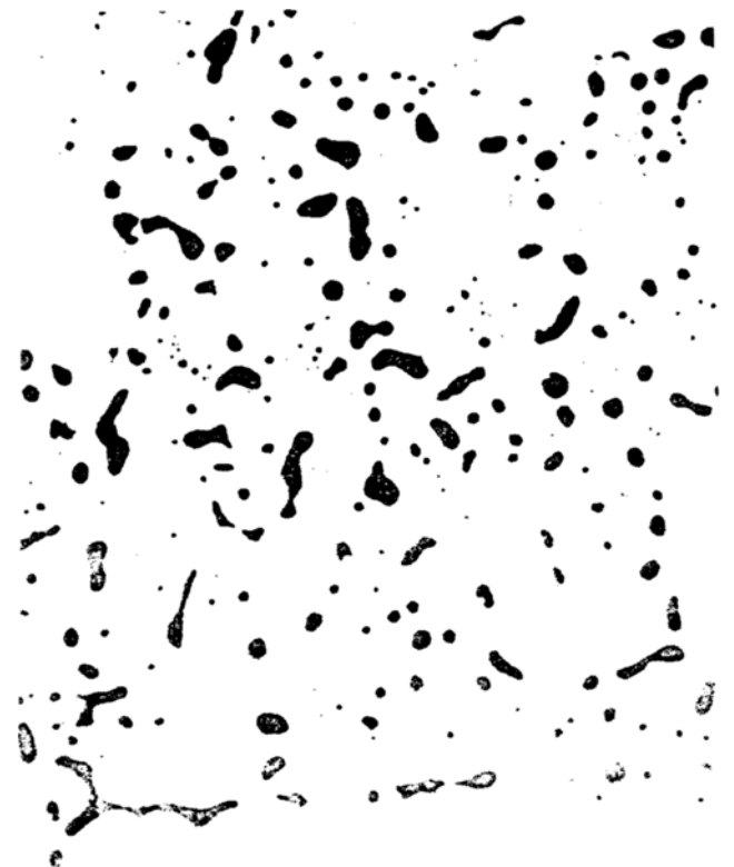
Fig. 9—Alloy 12. Degenerate rod morphology. 0.93 pct Mn, 1.3 pct S, Magnification 600 times.
