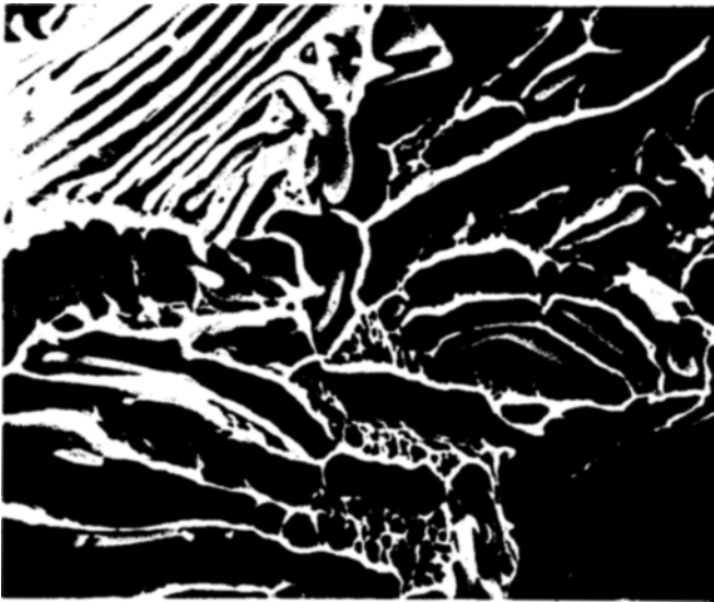
Fig. 19—Dominant Type IIR inclusions in fracture surface of Alloy 49. Scanning electron microscope picture. Magnification 1560 times.
