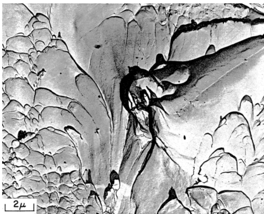
Fig. 7—Two-stage replica electron fractograph of Ti-10 at. pct Mo tensile specimen quenched from 950°C showing large shear-like features which are characteristic of this intermediate aging condition.
