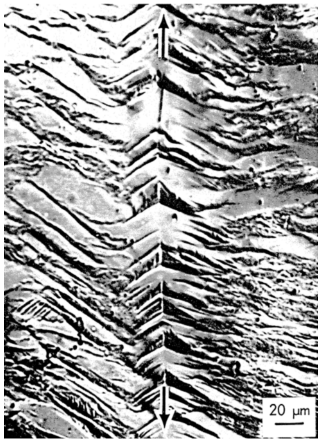
Fig. 2—Optical photomicrograph of stress-induced martensite revealed by its surface relief. Direction of applied stress is indicated by arrows. (Alloy 6811-15 after 80 pct reduction in thickness at 250°C.) Electropolished (90 pct/10 pct acetic/perchloric acid solution at 0°C and 20 V).
