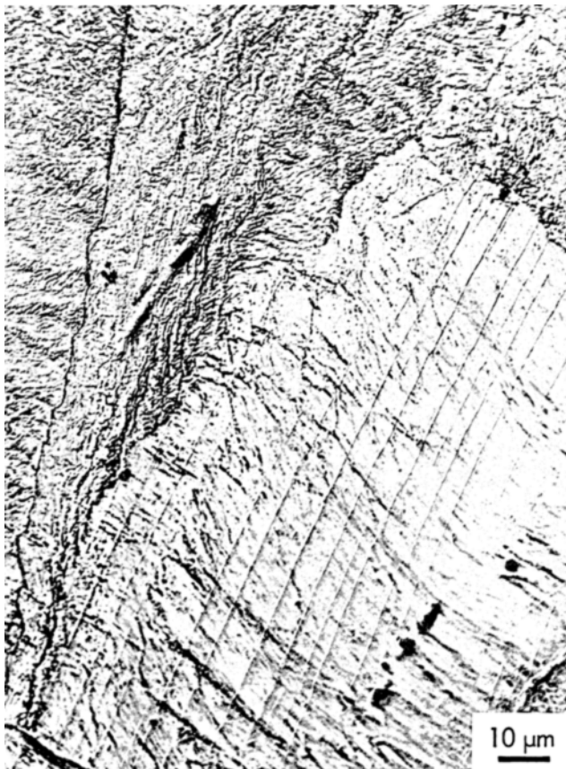
Fig. 1—Optical photomicrograph of the microstructure of Alloy 689-15 after 80 pct reduction in thickness at room temperature showing deformation markings in an austenitic grain that is surrounded by deformation-induced martensite. Electropolished (90 pct/10 pct acetic/perchloric acid solution at 0°C and 20 V) and etched (5 g cupric chloride, 100 ml hydrochloric acid, 100 ml methyl alcohol, and 100 ml distilled water).
