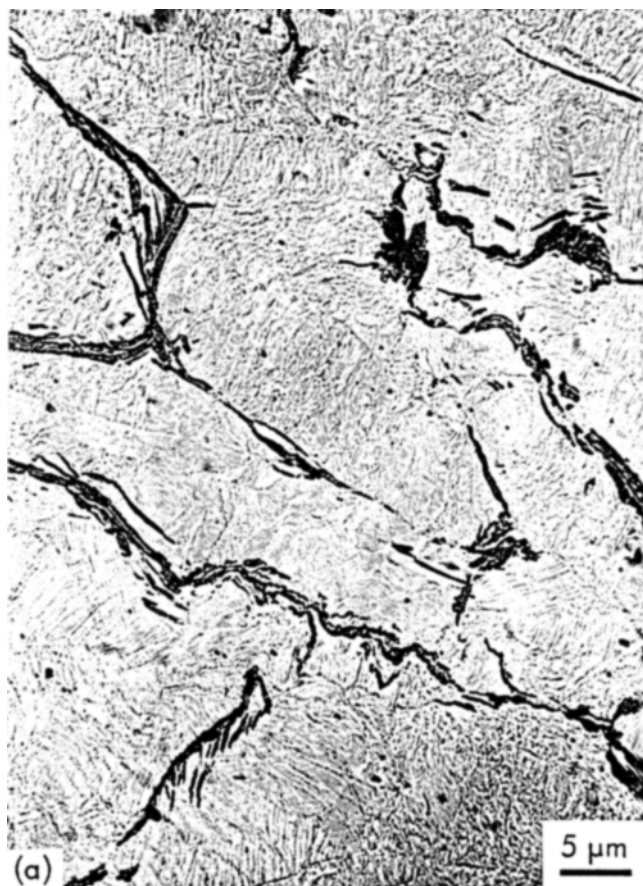
Fig. 17—Optical photomicrograph of the microstructure of Alloy 6811-13 after 60 pct reduction in thickness at 450°C (rolling time: 40 min). (a) Untempered; (b) tempered (80 min at 450°C). Electropolished (90 pct/10 pct acetic/perchloric acid solution at 0°C and 20 V) and etched (5 g cupric chloride, 100 ml hydrochloric acid, 100 ml methyl alcohol, and 100 ml distilled water).
