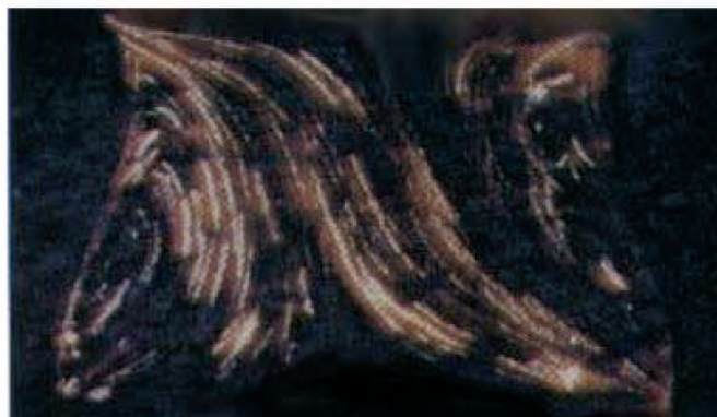
Fig. 6 Photograph of Oscillatory Thermocapillary Flow for Ar = 0.6 at T_R = +23^\circ\text{C} .
